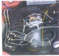
in-line, and placed with its center of gravity in front of the axle. Fuel injection is CIS (Continuous Injection System), which contributes to smooth performance and efficient use of fuel, as well as clean exhaust emission. Because it has CIS instead of carburetion, The Fox excels at cold-weather starting.
