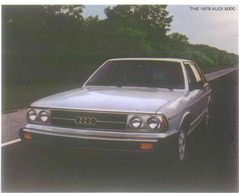
All Audis are designed with a type of body construction that places a rigid "passenger cell" between two impact areas, or "crumple zones," front and back which absorb the energy of a crash while the passenger cell remains intact.
